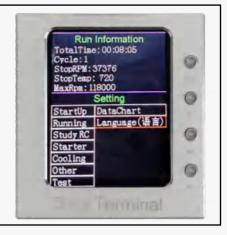
select 'ad just temp' and click '+-' to adjust the temperature up and down, keeping the corrected temperature consistent with the ambient temperature.
