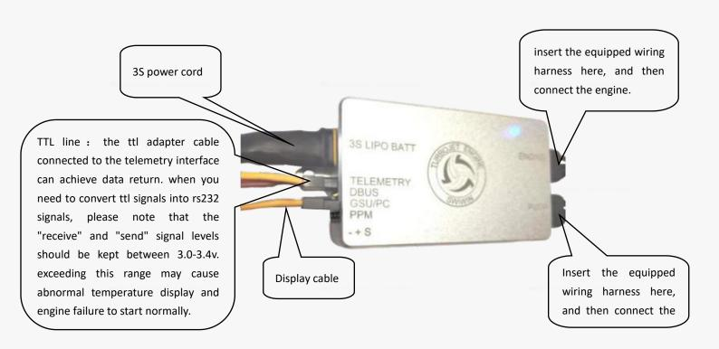
the ttl serial port control method can achieve computer control of the engine.
